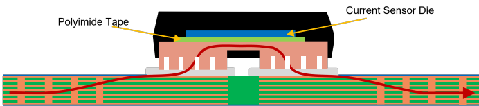
Figure 5: No Vias Under Copper Pads Example
