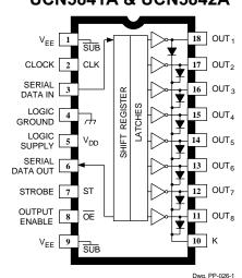
Note that the UCN584xA (dual in-line package) and UCN584xLW (small-outline IC package) are electrically identical and share a common terminal number assignment.
