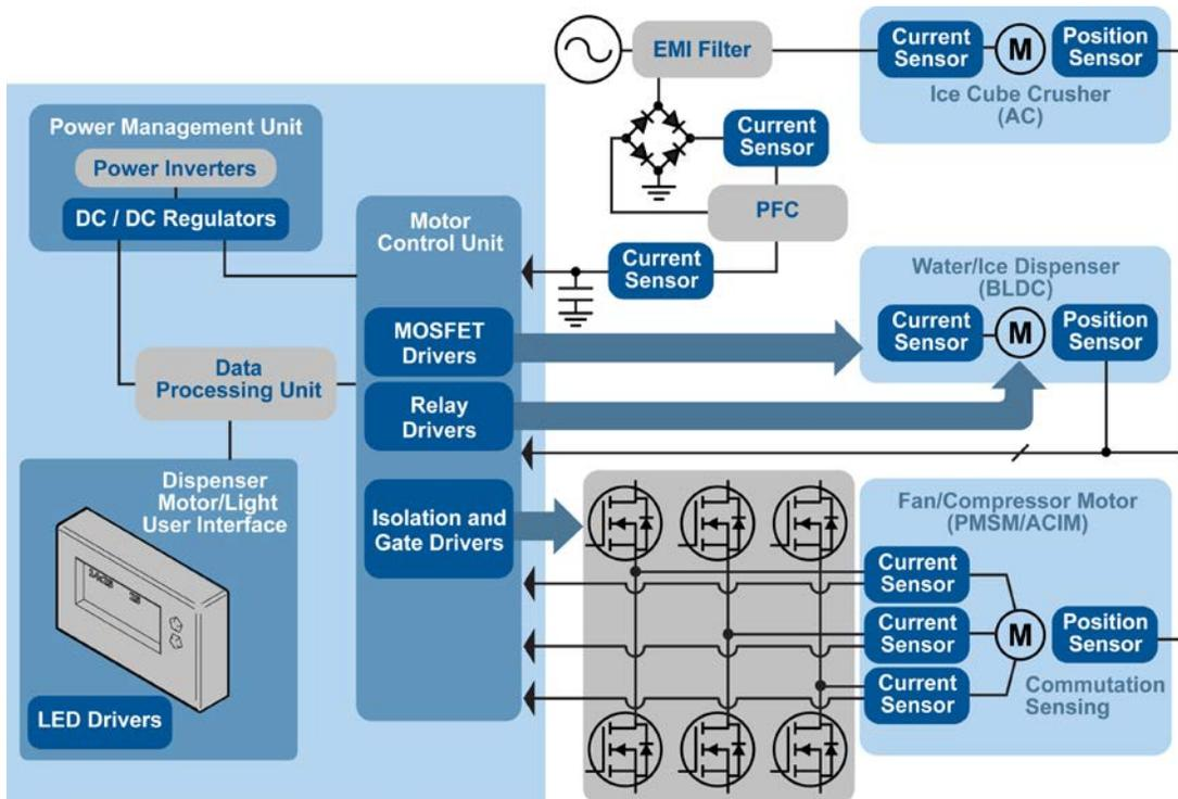
Allegro's integrated Hall current sensor IC portfolio delivers performance features that meet a wide range of requirements for motor control that are critical to a refrigerator's energy efficiency, safety and reliability requirements.
