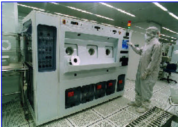
Wafer Cleaning: Semi-automated wafer cleaning at all diffusion operations using state-of-the-art chemistry resulting in low particulate and metallic levels.
