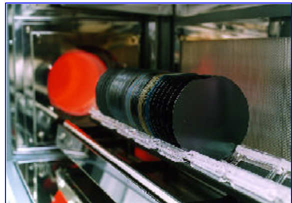
Diffusion: Automated diffusion tubes with cantilever load, computerized control and recipe management, and external torch assemblies.
