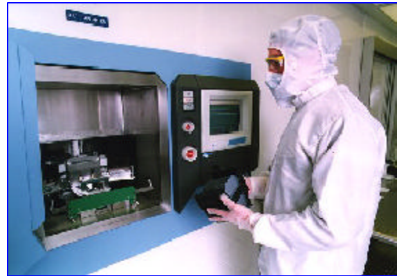
Ion Implant: State-of-the-art high current implanter capable of the full range of dose requirements.
