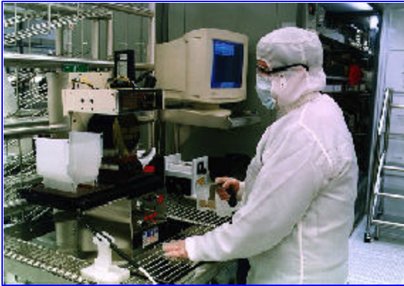
Wafer Loading: Automated wafer loading throughout the Fab prevents handling-induced mechanical damage.
