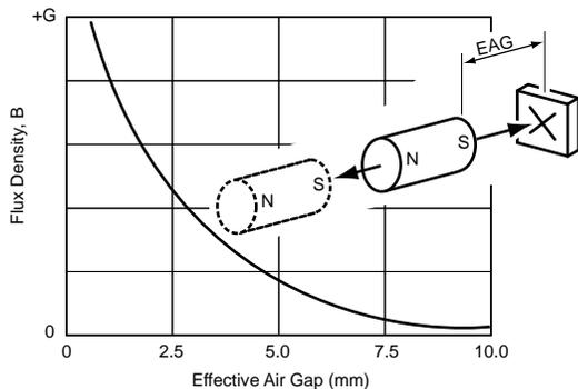
Figure 8. Head-on application configuration and response curve, showing a monotonic characteristic regardless of pole orientation.
