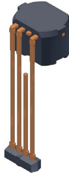
Figure 21. SG package after pin 3 trimming, and bending remaining pins
