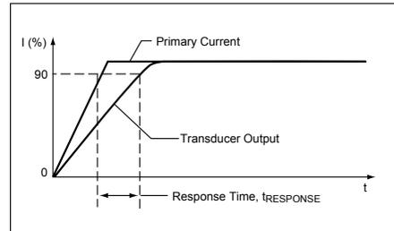
**Rise time ( $t_r$ ).** The time interval between a) when the device reaches 10% of its full scale value, and b) when it reaches 90% of its full scale value. The rise time to a step response is used to derive the bandwidth of the device, in which  $f(-3\text{ dB}) = 0.35/t_r$ . Both  $t_r$  and  $t_{RESPONSE}$  are detrimentally affected by eddy current losses observed in the conductive IC ground plane.
