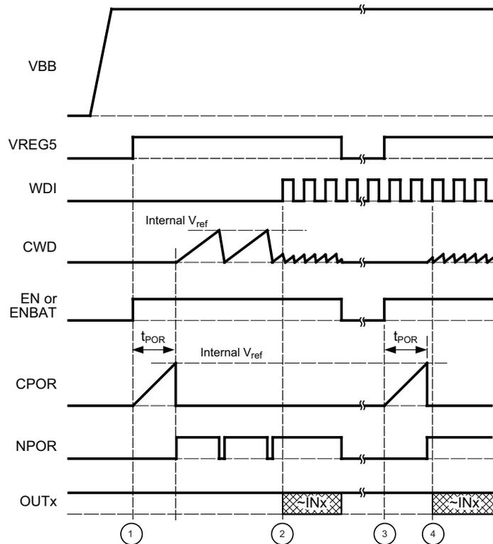
1. 5 V signal to wake up microcontroller.
