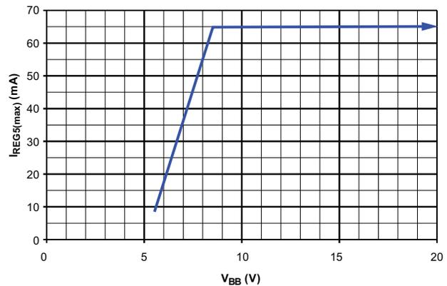
Figure 3. Current Capability of the 5 V Regulator (VREG5)
