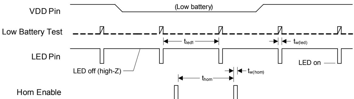
**Local Smoke Detection/Test Alarm Condition**
