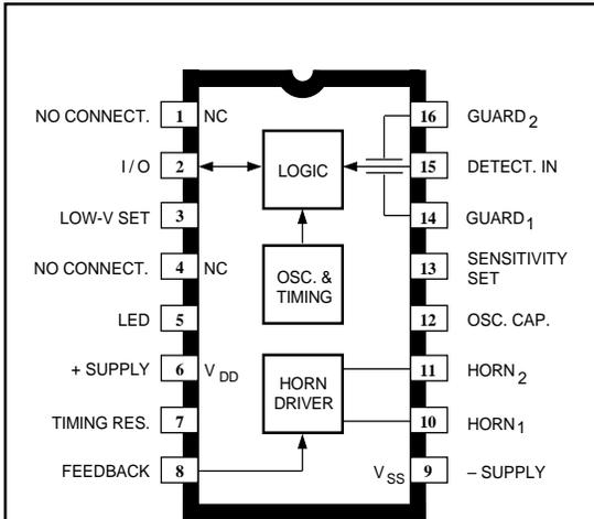
The A5354CA is a low-current, CMOS circuit providing all of the required features for an ionization-type smoke detector. A networking capability allows as many as 125 units to be interconnected so that if any unit senses smoke, all units will sound an alarm. In addition, special features are incorporated to facilitate alignment and test of the finished smoke detector. This device is designed to comply with Underwriters Laboratories Specification UL217.
