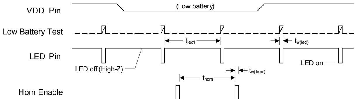
**Local Smoke Detection/Test Alarm Condition**
