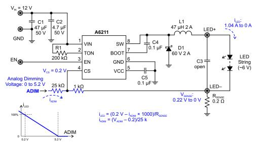
Figure 17: Analog Dimming of LED Current with an External DC Voltage
