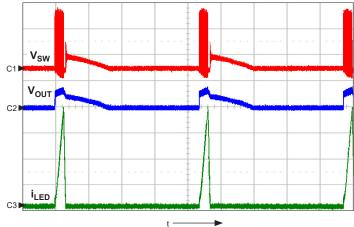
Figure 10: A6211 overcurrent protection tripped in the case of a fault caused by the sense resistor pin shorted to ground; shows switch node,  $V_{SW}$  (ch1, 10 V/div.), output voltage,  $V_{OUT}$  (ch2, 10 V/div.), LED current,  $i_{LED}$  (ch3, 1 A/div.), t = 100 µs/div.
