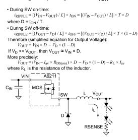
$$t_{ON} = k \times (R_{ON} + R_{INT}) \times (V_{OUT} / V_{IN})$$
