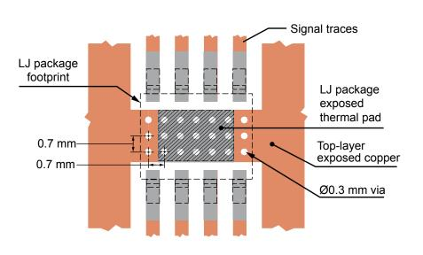
Figure 21: Suggested PCB Layout for Thermal Optimization (Maximum Available Bottom-Layer Copper Recommended)
