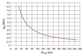
Figure 6: Switching Frequency versus R<sub>TON</sub> Resistance
