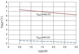
Figure 9: Minimum and Maximum Output Voltage versus  $i_{LED}$  current (V<sub>IN</sub> = 9 V,  $f_{SW}$  = 1 MHz, minimum  $t_{ON}$  and  $t_{OFF}$  = 150 ns)
