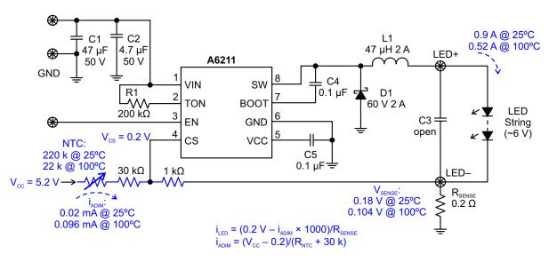
Figure 18: Thermal Foldback of LED Current using NTC Resistor
