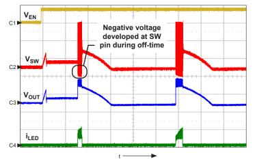
Figure 11: Startup waveform with a missing Schottky diode; shows Enable,  $V_{EN}$  (ch1, 5 V/div.), switch node,  $V_{SW}$  (ch2, 5 V/div.), output voltage,  $V_{OUT}$  (ch3, 5 V/div.), LED current,  $i_{LED}$  (ch4, 500 mA/div.), t = 100 µs/div.
