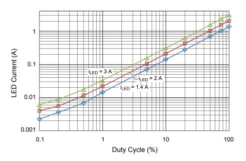
Figure 5: Average LED Current versus PWM dimming percentage Operating conditions: V<sub>IN</sub> = 12 V, V<sub>OUT</sub> = 3.5 V, f<sub>SW</sub> = 1 MHz, f<sub>PWM</sub> = 200 Hz, L = 10  $\mu$ H
