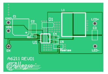
Figure 19: Example Layout for the A6211 Evaluation Board
