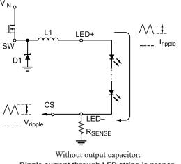
Ripple current through LED string is proportional to ripple voltage at CS pin.
