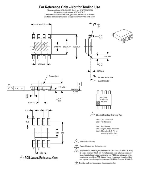
Figure 22: Package LJ, 8-Pin Narrow SOIC with Exposed Thermal Pad
