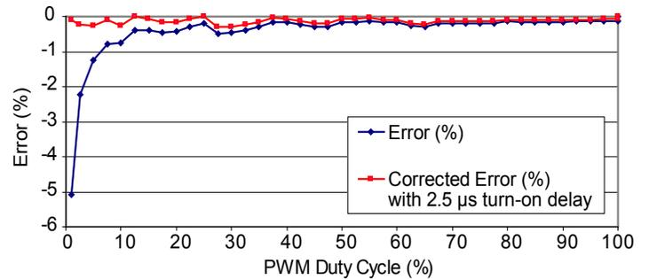
The LED Current Error graph shows the effect of PWM duty cycles on LED current error, according to the relationship:
