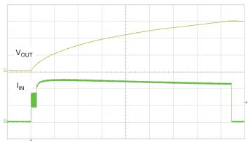
$V_{BAT}$  = 2 V. C1,  $V_{OUT}$  100 V/div; C4,  $I_{IN}(av)$  200 mA/div; Time 1s/div.
