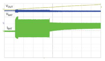
Figure 12. Input current waveforms with Li+ battery connected by 5-in. wire and decoupled by 4.7  $\mu$ F capacitor. C1, V<sub>OUT</sub> 100 V/div; C3, V<sub>BAT</sub> 2 V/div; C4, I<sub>BAT</sub> 500 mA/div; Time, 50 ms/div.
