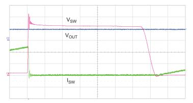
Figure 5. Zero-Voltage Switching (ZVS)  $V_{BAT}$  = 3.6 V,  $I_{SWlim}$  = 1.2 A. C2,  $V_{SW}$  = 2 V/ div; C3,  $V_{OUT}$  = 50 V; C4,  $I_{SW}$  = 500 mA/div; Time = 0.5 µs/div.
