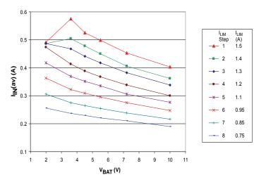
Note: Peak switch current is limited by maximum on-time and di/dt of transformer primary current; therefore, average current drops at very low battery voltage.
