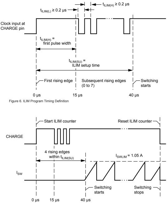
Figure 7. Current Limit Programming Example (Iswim4 selected)
