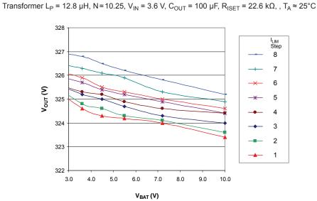
Final Output Voltage versus Battery Voltage Transformer L = 12.8 µH N=10.25 V № = 3.6 V Court = 100 µE Right = 22.6 kO Ta ≈ 25°
