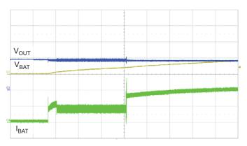
Figure 14. Input current waveforms with Li+ battery connected through 10  $\mu$ H inductor and 10  $\mu$ F capacitor. C1, V<sub>OUT</sub> 100 V/div; C3, V<sub>BAT</sub> 2 V/div; C4, I<sub>BAT</sub> 200 mA/div; Time, 50 ms/div.
