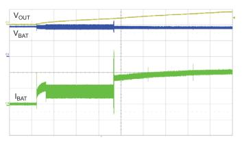
Figure 13. Input current waveforms with Li+ battery connected through 10  $\mu$ H inductor and 4.7  $\mu$ F capacitor. C1, V<sub>OUT</sub> 100 V/div; C3, V<sub>BAT</sub> 2 V/div; C4, I<sub>BAT</sub> 200 mA/div; Time, 50 ms/div.
