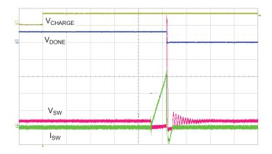
Figure 9. Operation under open diode fault ( $I_{SWlim} = 1.5 \text{ A}, V_{BAT} = 3.6 \text{ V}, L_{primary} = 12.8 \mu\text{H}$ ). C1,  $V_{CHARGE}$ , 5 V/div; C2,  $V_{SW}$  10 V/div; C3,  $\overline{\text{DONE}}$  5 V/div; C4,  $I_{SW}$  500 mA/div; Time, 10 µs/div.
