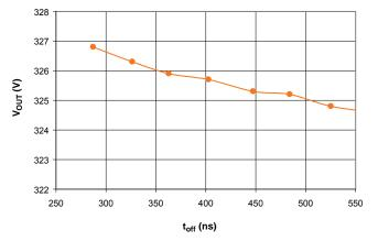
The value of t<sub>off</sub> depends on I<sub>SWlim</sub>, primary inductance, L<sub>Primary</sub>, and turns ratio, N, as given by:  $t_{off} = (I_{SWlim} \times L_{Primary} \times N) / V_{OUT}$ .
