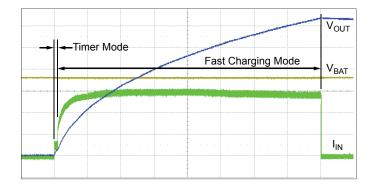
Figure 3. Timer mode and Fast Charging mode: t = 200 ms/div;  $V_{OUT}$  = 50 V/div;  $V_{BAT}$  = 1 V/div.;  $I_{IN}$  = 100 mA/div.,  $V_{BAT}$  = 3.6 V;  $C_{OUT}$  = 20 µF/330 V; and  $I_{SWlim} \approx 0.75$  A.
