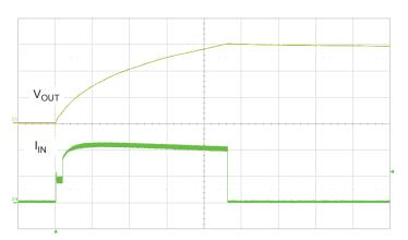
$V_{BAT}$  = 3.6 V. C1,  $V_{OUT}$  100 V/div, C4;  $I_{IN}(av)$  200 mA/div; Time 1s/div.
