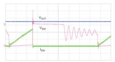
Figure 4. Expanded view of Timer Mode, V<sub>BAT</sub> = 3.6 V, I<sub>SWlim</sub> = 1.2 A. C2, V<sub>SW</sub> = 2 V/div; C3, V<sub>OUT</sub> = 50 V/div; C4, I<sub>SW</sub> = 500 mA/div; Time = 2 µs/div.
