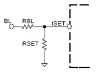
Figure 8. Optional Smart Current Limit configuration
