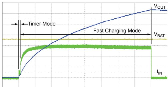
Figure 5. Timer Mode and Fast Charging Mode.  $t = 200 \text{ ms/div}$ ,  $V_{OUT} = 50 \text{ V/div}$ ,  $V_{BAT} = 1 \text{ V/div}$ ,  $I_{IN} = 100 \text{ mA/div}$ ,  $V_{BAT} = 3.6 \text{ V}$ ,  $C_{OUT} = 20 \mu F/330 \text{ V}$ ,  $R_{SET} = 46 \text{ k}\Omega$  ( $I_{SWlim} \approx 0.75 \text{ A}$ ).
