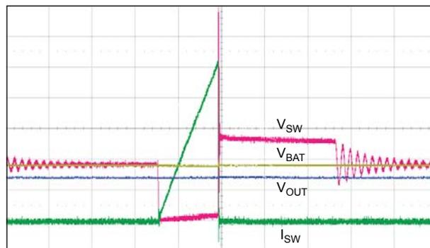
Figure 6. Timer Mode expanded view.  $V_{OUT} \leq 14 \text{ V}$ ,  $t = 2 \mu s / \text{div}$ ,  $V_{BAT} = 3.6 \text{ V}$ ,  $R_{SET} = 33.2 \text{ k}\Omega$ .
