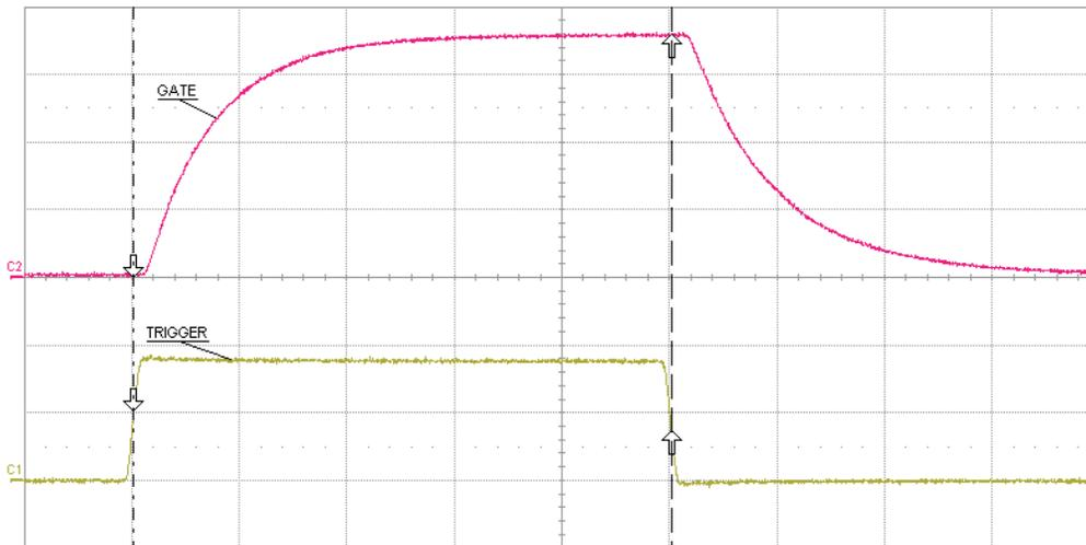
$C_{GATE} = 6200 \text{ pF}$ ,  $V_{IN} = 3.6 \text{ V}$ , Time = 200 ns/div; CH1 = TRIGGER input, 2 V/div,
