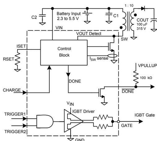
Figure 1. Typical application with separate trigger inputs.
