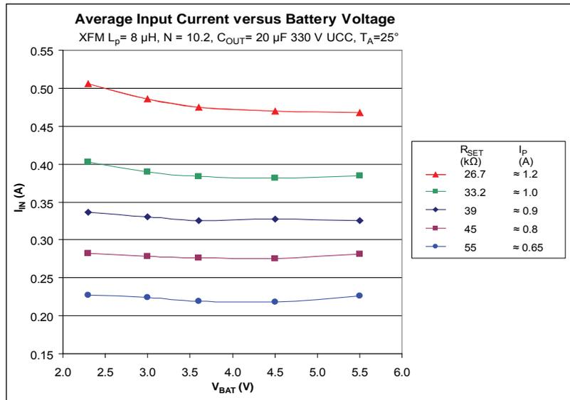
An increase in  $I_{SWlim}$  with respect to  $V_{BAT}$  actually keeps the average input current roughly constant throughout the battery voltage range. Normally, if  $I_{SWlim}$  is kept constant, the average current will drop as  $V_{BAT}$  goes higher.
