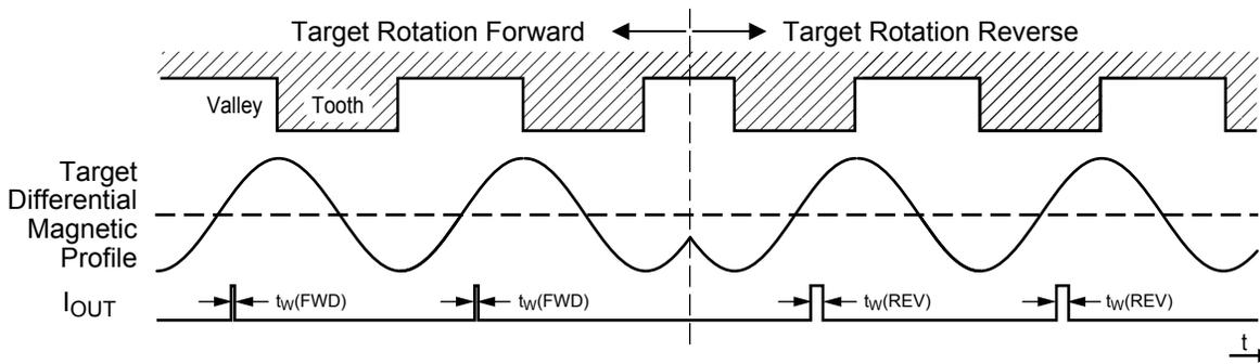
Figure 5. Example of direction change in Running mode
