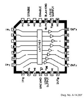
Information present at an input is transferred to its latch when the STROBE and ENABLE are high. The latches will continue to accept new data as long as both STROBE and ENABLE are held high. With either STROBE or ENABLE in the low state, no information can be loaded into the latches.
