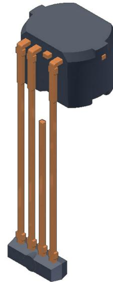
Figure 20. SG package after pin 3 trimming, and bending remaining pins
