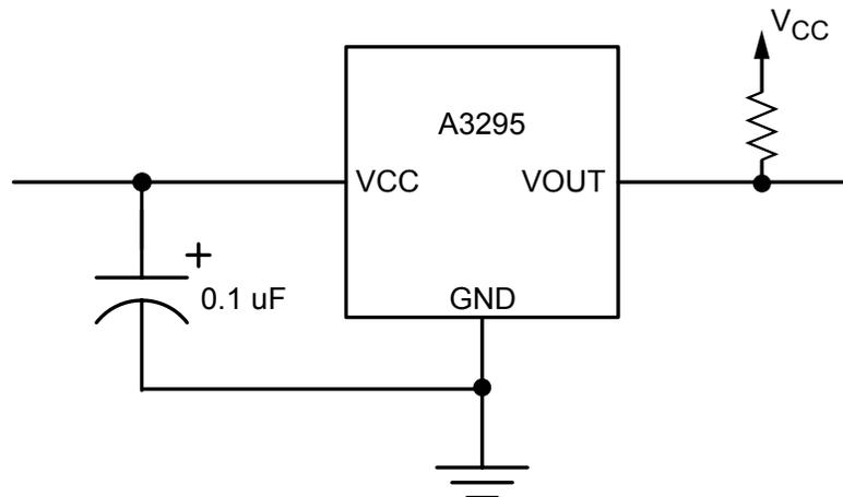
**Figure 4: Typical Basic Application Circuit**
