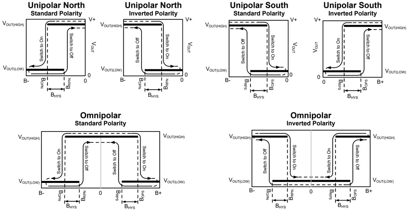
Figure 1: Hall switch magnetic and output polarity options
