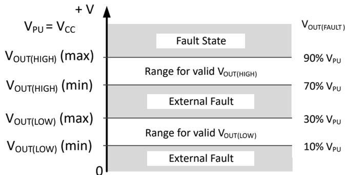
Figure 6: APS11450 valid (typical) and fault-condition output levels
