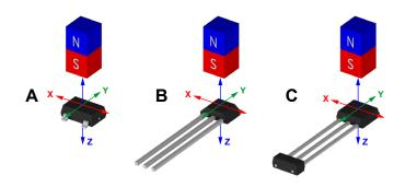
Figure 2: Magnetic Sensing Orientations APS12400 LH (Panel A), UA (Panel B), and UC (Panel C)
