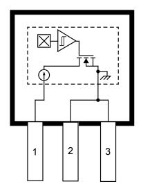
LH Package, 3-Pin SOT23W Pinout
