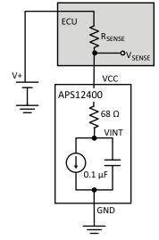
(D) High-Side Sensing (UC package)
