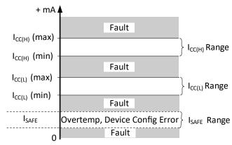
Figure 4: Interpreting I<sub>CC</sub> for System-Level Diagnostics
