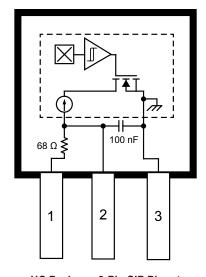
UC Package, 3-Pin SIP Pinout
