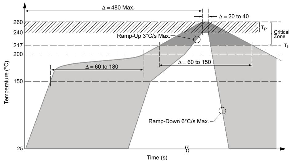
Figure 9. Solder Reflow Profile for SMD Using Lead (Pb) Free Solder. The typical acceptable maximum temperature range,  $T_P$ , is 240°C to 260°C. Temperatures refer to upper surface of the package case.
