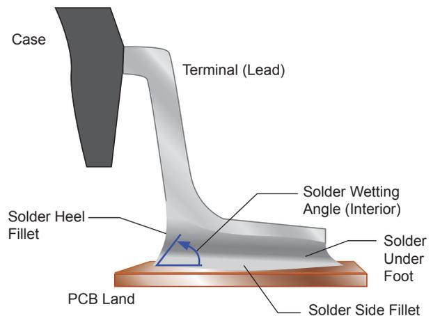
**Figure 5. Gull Wing Solder Joint.** Under optimum conditions, a smooth, concave fillet at the heel and sides can be observed. A solder layer between the terminal foot and the land is critical. A low wetting angle is expected between the edge of the solder and the terminal and land surfaces.
