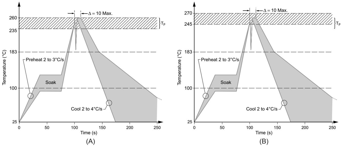
Figure 10. Solder Profile for Through-Hole Wave Solder Using (A) Traditional Tin-Lead Solder and (B) Pb-free solder.
