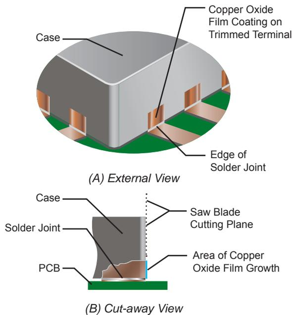
Figure 3. QFN and SON Solder Joints. The saw blade cut or scored break edge leaves exposed copper in those designs where the terminal material extends to the edge of the package case after singulation.
