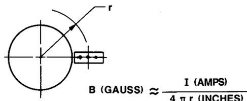
Note that the Hall element is most sensitive to magnetic fields passing perpendicularly through it. Flux lines at an angle to the device will generate reduced (cosine of the angle) Hall voltages and flux lines at  $90^{\circ}$  angles will produce a zero gauss indication.
