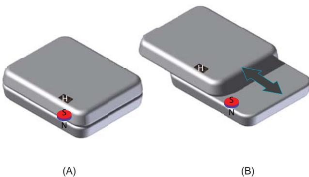
Figure 1. Hall-effect sensor IC and magnet positions on a standard slide phone
