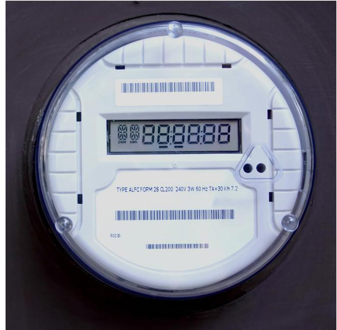
**Figure 1: Typical Smart Electric Meter**
