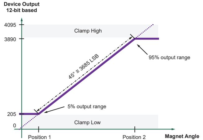
**Figure 8: Clamps and output range limitation – short stroke on 45° using 90% of output range**
