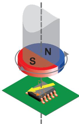
**Figure 1: Sensor and magnet orientation – end of shaft**
