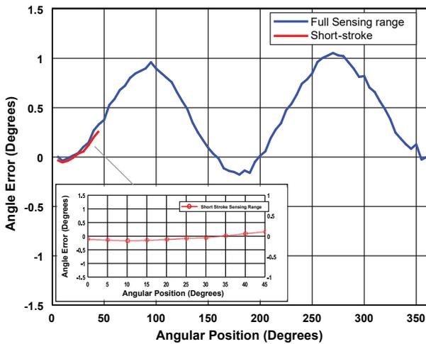
**Figure 5: Angle error on full sensing range vs. stroke range**
