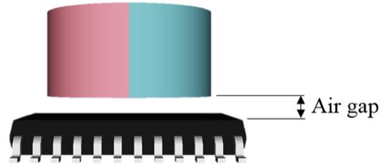
**Figure 2: Air gap definition**
