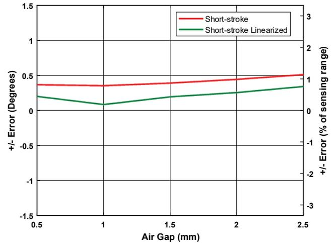
**Figure 11: Accuracy error across air gap with and without linearization – short-stroke range**
