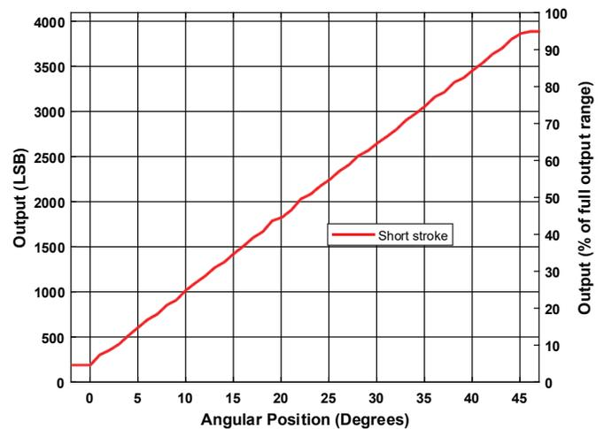
**Figure 9: Device output with 45° short stroke limited to 90% of output range**
