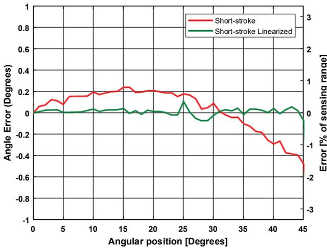
**Figure 10: Short-stroke angle error at 1 mm air gap, with and without linearization**
