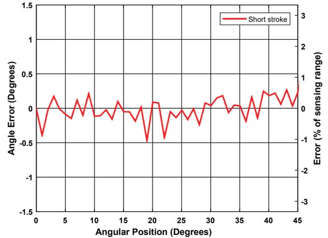
**Figure 6: Short stroke angle error at 0.5 mm air gap**
