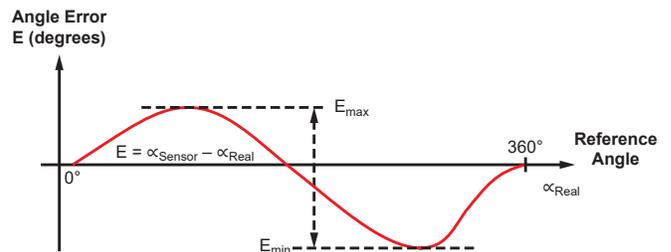
**Figure 3: Angle error definition**
