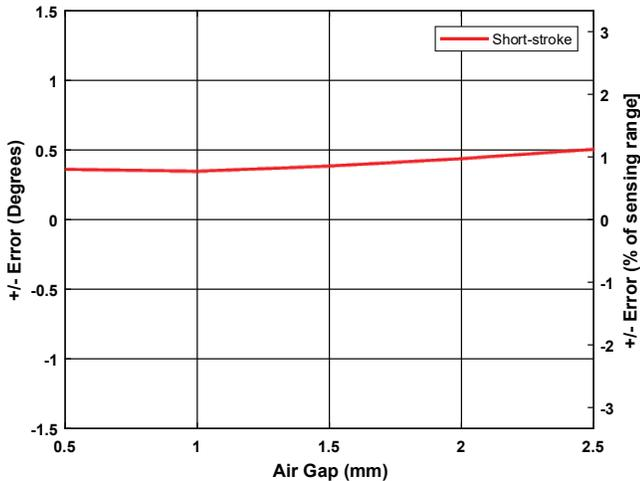
**Figure 7: Short stroke accuracy error across air gap**
