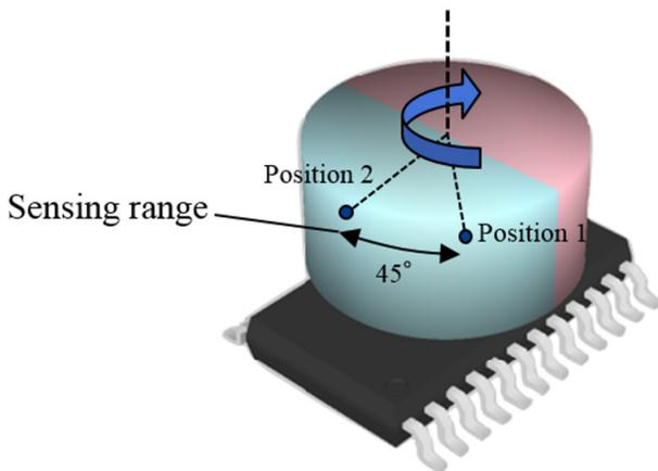
**Figure 4: Short stroke range on 6 mm × 4 mm magnet and dual die device (TSSOP-24 package)**
