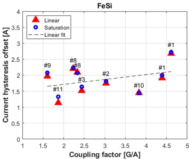
Figure 8: Current hysteresis offset versus coupling factor for FeSi cores
