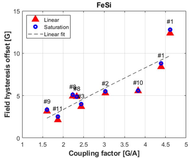
Figure 7: Field hysteresis offset versus coupling factor for FeSi cores
