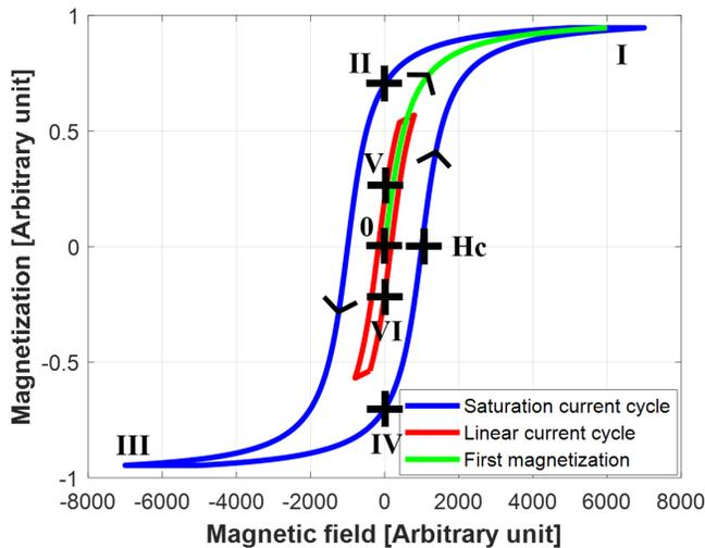
Figure 2: Schematic behavior of a soft ferromagnetic material
