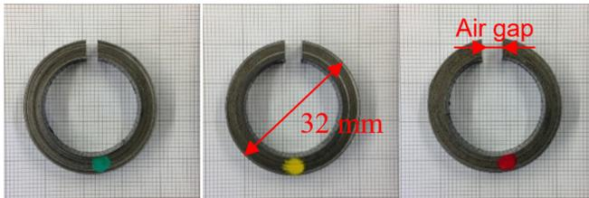
Figure 4: Photos of cores #1, #2, and #3 (from left to right)
