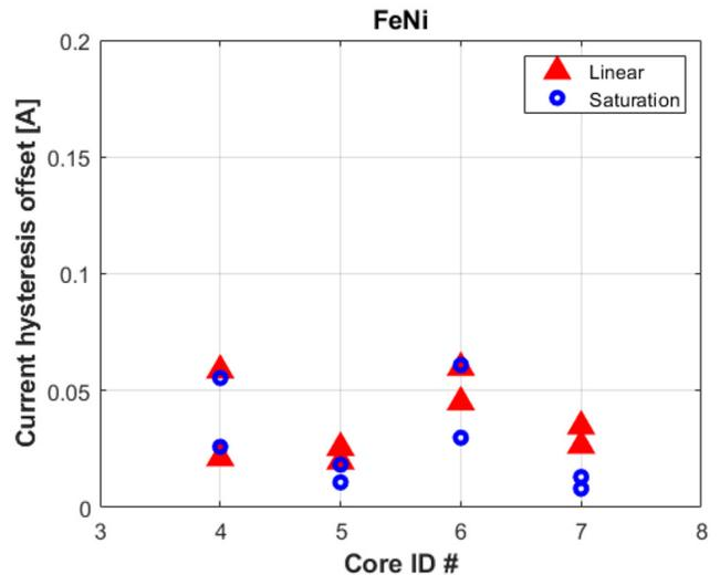
Figure 9: Current hysteresis offset for FeNi cores
