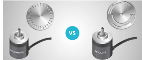
Figure 3: Incremental Encoding vs. Absolute Encoding Example [5]
