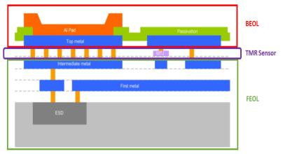
Figure 9: XtremeSense TMR construction
