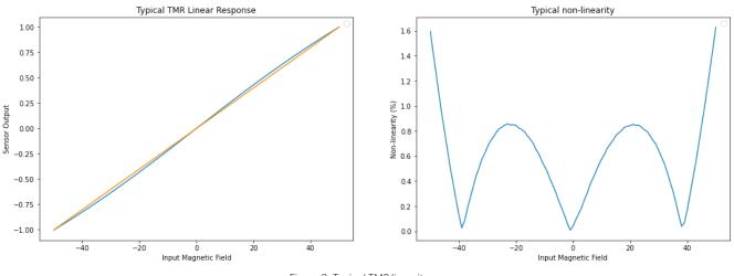
Figure 2: Typical TMR linearity error
