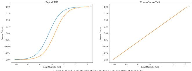
Figure 4: Magnetic hysteresis of typical TMR devices vs XtremeSense TMR
