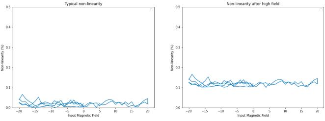
Figure 7: Offset in nonlinearity after contact with magnetic field
