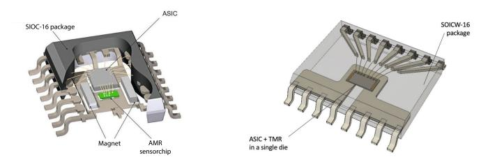
Figure 10: Multi-die package solution versus single-die package solution with XtremeSense TMR
