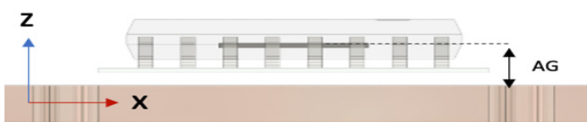
Figure 5: Side-View of CTD452/3 on Top of Busbar
