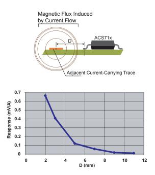
Figure 4. Adjacent Conduction Traces Carrying 50 A, Effect on an ACS71x device. The minimal influence of magnetic effects from an adjacent trace diminish rapidly as the distance, D, is increased.
