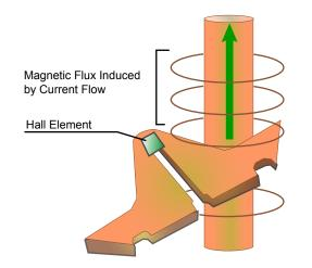
Figure 3. Adjacent Conduction Perpendicular to Hall Element Plane. Flux lines generated perpendicular to current flow are parallel to Hall plane and do not generate Hall voltage.
