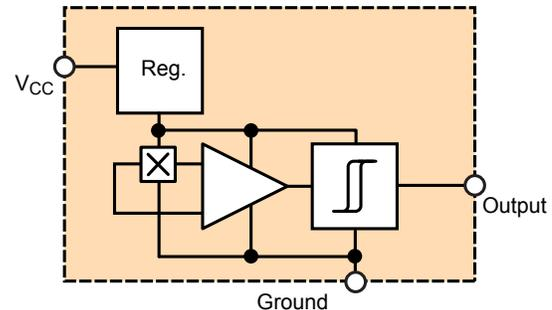
Figure 6. Hall circuit with digital output capability
