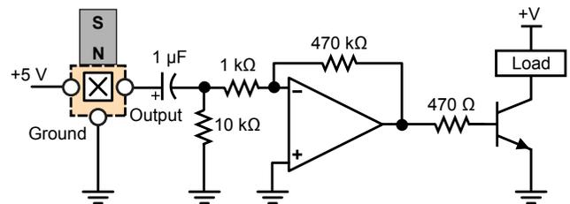
Figure 70. Typical external back-biasing application circuit to detect the absence of a ferromagnetic target
