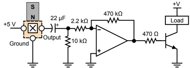
Figure 68. Typical external back-biasing application circuit to detect absence of target
