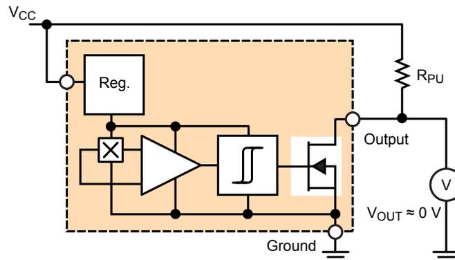
Figure 11. Test circuit for transfer characteristic charts
