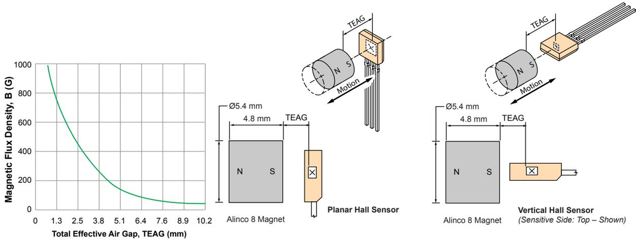
Figure 12B. Demonstration of head-on mode of operation
