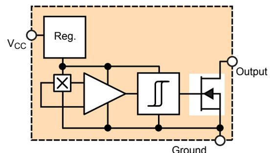
Figure 7. Common circuit elements for Hall switches
