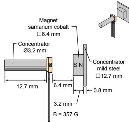
Figure 58A. Effect of 12.7 mm<sup>2</sup> additional flux concentrator, attached to magnet
