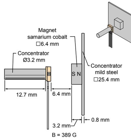
Figure 58B. Effect of 25.4 mm<sup>2</sup> additional flux concentrator, attached to magnet
