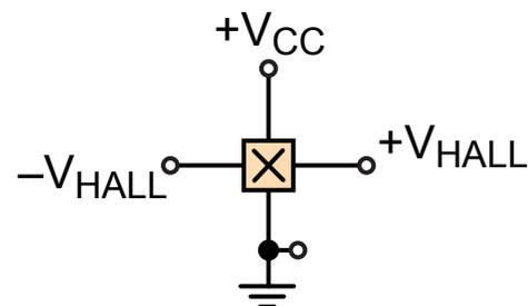
Figure 1. Schematic representation of the active area of a Hall-effect device, with the Hall element represented by the component marked with an X.
