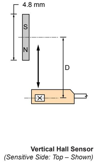
Figure 51. Example of slide-by motion, magnet on one side, single magnet
