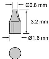
Figure 72. Printer drum sensing application flux concentrator
