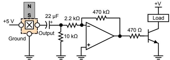
Figure 69. Typical external back-biasing application circuit to detect the presence of a ferromagnetic target
