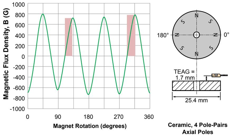
Figure 24. Magnetic flux characteristic of a ring magnet
