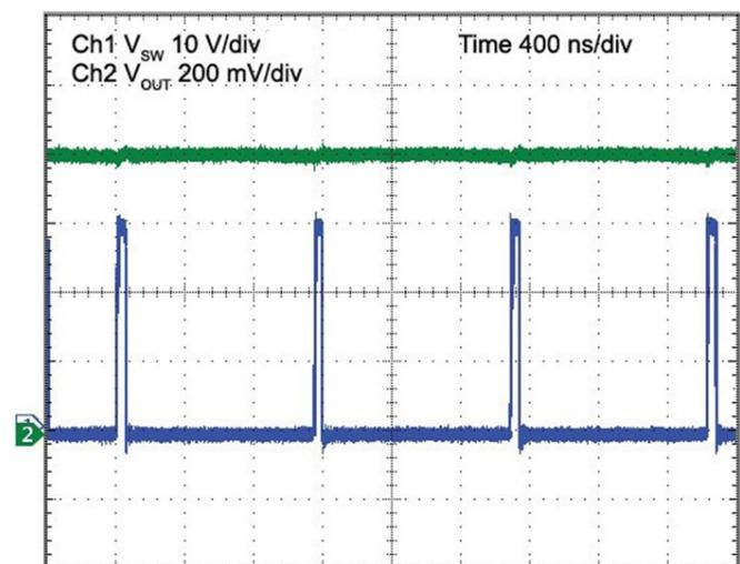
Figure 4: Duty cycle less than 6%; no pulse skipping.
