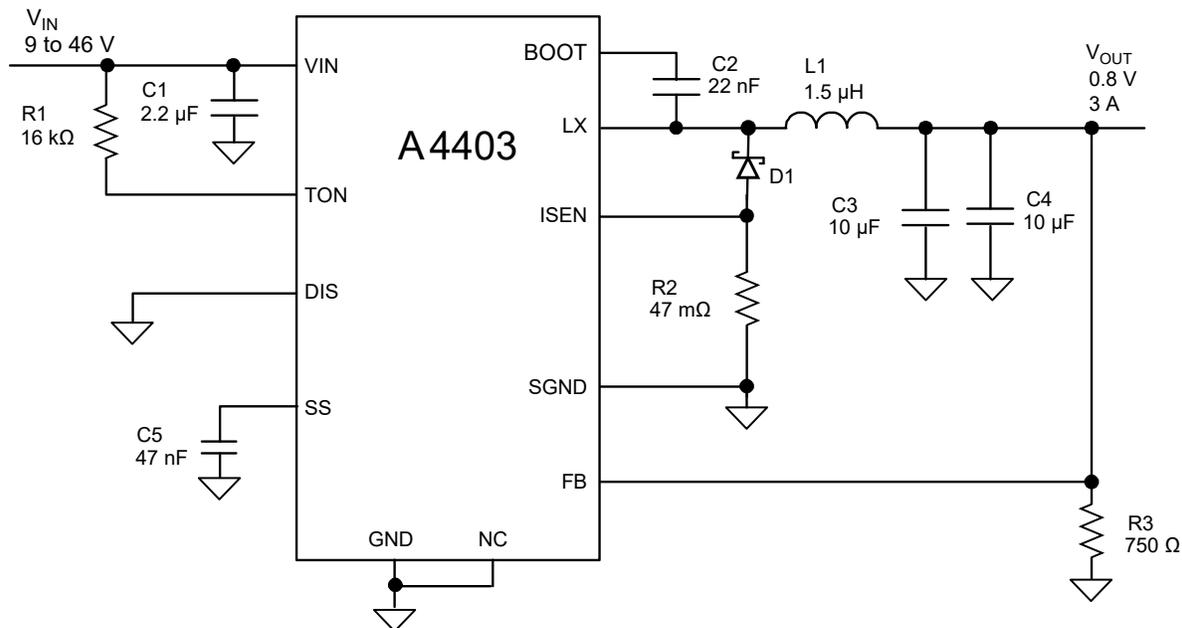
Figure 5: Typical application using the A4403.
