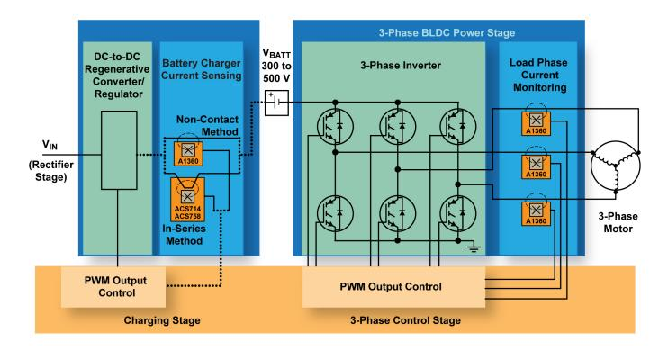
Figure 3. (Left): DC-DC Converter Charger, and (right): Three-Phase DC-AC Inverter
