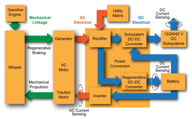
Figure 1. Typical HEV System Block Diagram
