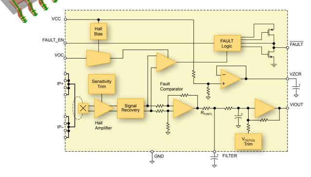
Figure 3. ACS710 current sensor IC in an SOIC16 package with block diagram
