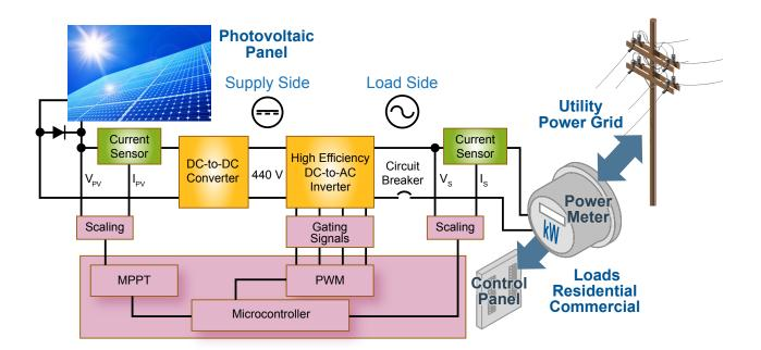
Figure 1. Photovoltaic system diagram
