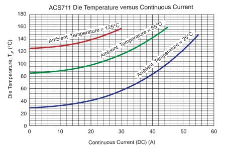
Figure 4. QFN Current Sensor Linear Thermal Performance on PCB
