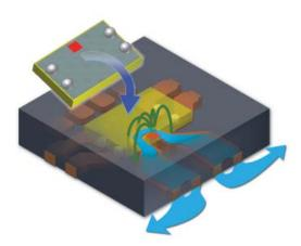
Figure 2. QFN Package Construction
