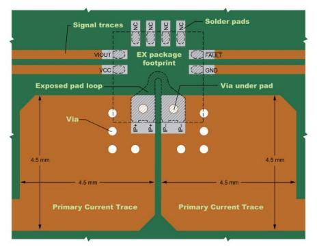
Figure 3. PCB Layout for QFN Current Sensor
