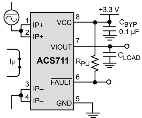
Figure 5. Typical application circuit for the ACS711
