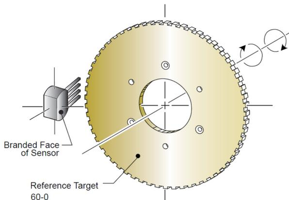
Figure 1: Magnetic Encoder Diagram
