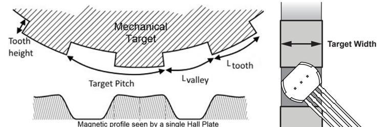
Figure 5: Target Parameters
