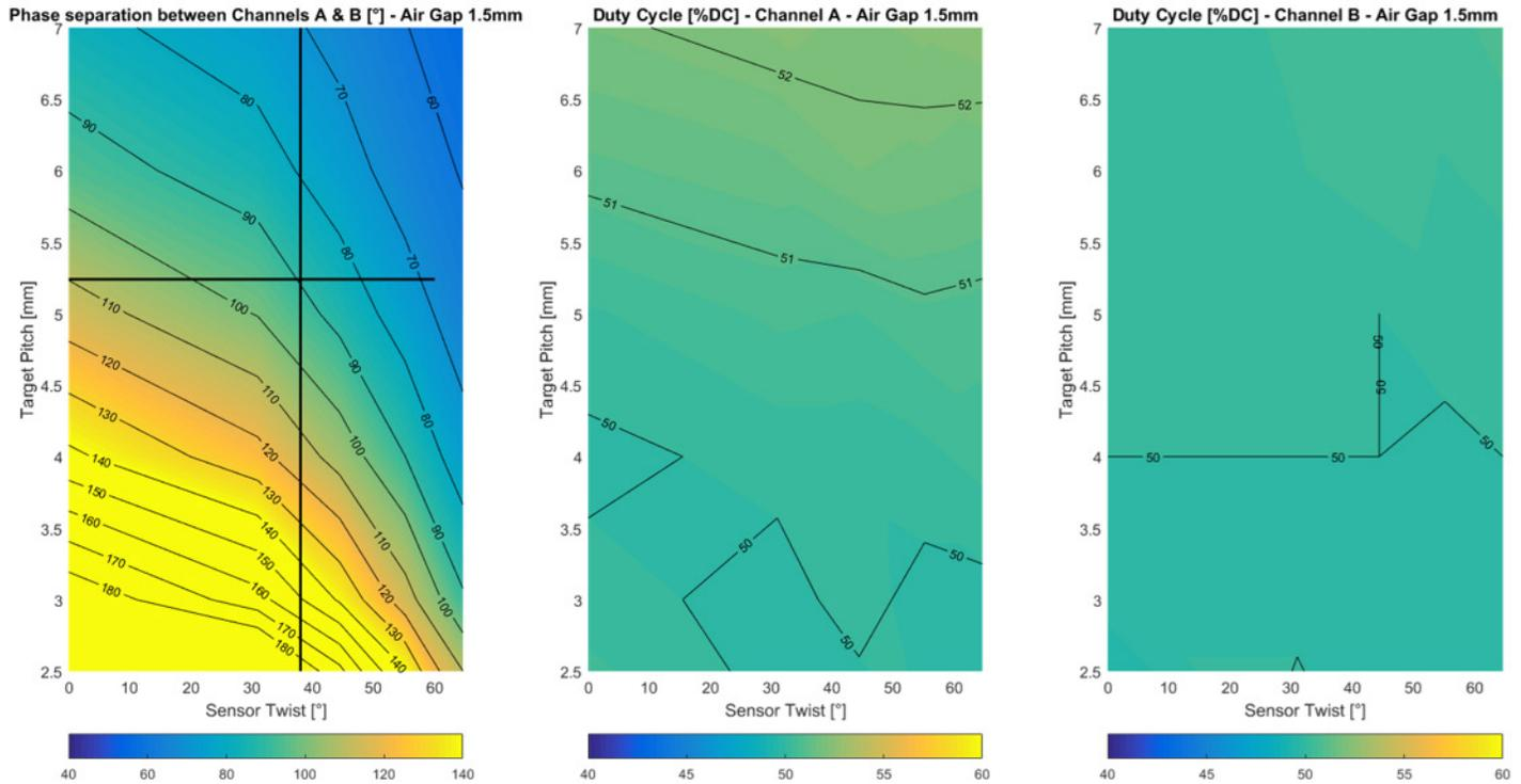
Figure 11: Sensor Twist over Target Pitch with Air Gap of 1.5 mm and Tooth/Pitch Ratio of 0.4
