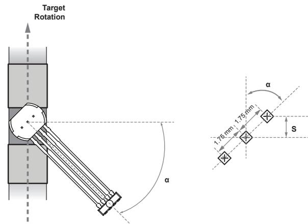
Figure 10: Sensor Twist in Front of the Target
