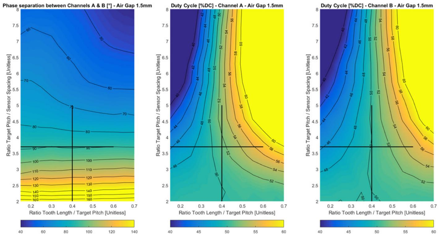
Figure 6: Phase Shift and Duty Cycle at 1.5 mm
