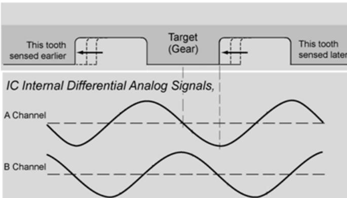
Figure 4: Differential Signals Sensed by the Sensor
