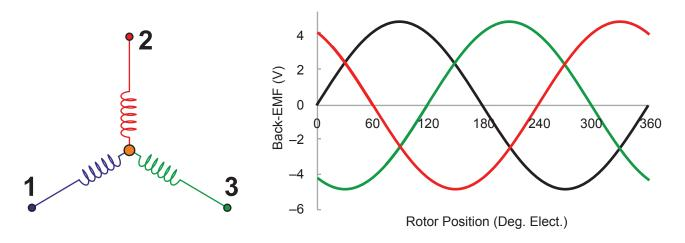
Back-EMF Frequency and Amplitude  $\alpha$  motor RPM. (Motor BEMF frequency and amplitude are both proportional to motor RPM.)
