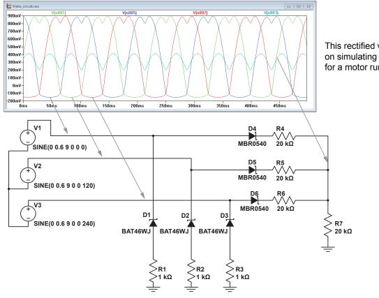
This rectified voltage is based on simulating BEMF signals for a motor running at ~100 RPM.
