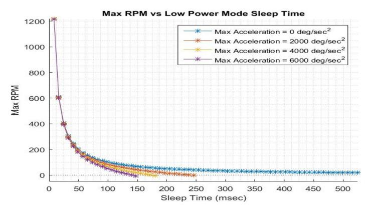
Figure 6: Maximum RPM versus Sleep Time
