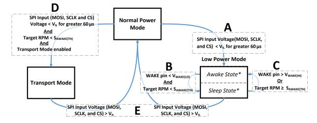
Figure 5: Operating Mode State Diagram
