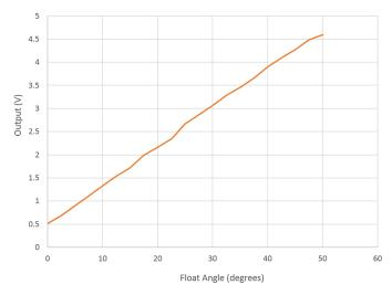
Figure 11: Float Angle vs. Output Voltage
