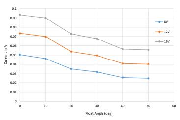
Figure 9: Float Angle vs. Coil Current
