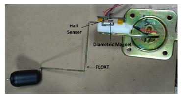
Figure 6: Arrangement of Hall Sensor and Magnet on the Fuel Sensor Assembly
