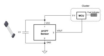
Figure 10: Linear Analog Hall-Effect Sensor-Based Digital FLS Using A1377
