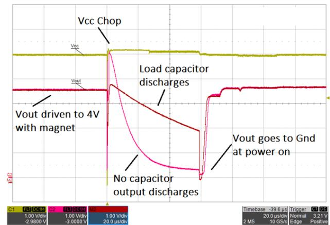
Figure 10: Capacitor discharge as part resets
