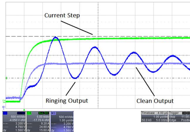
Figure 4: Clean trace overlaid with ringing trace
