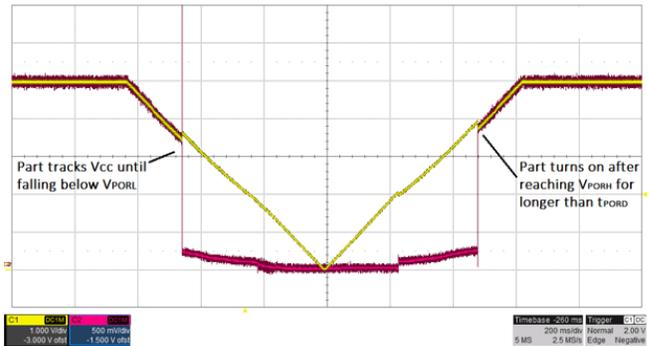
Figure 9: Part output during slow V<sub>CC</sub> ramp
