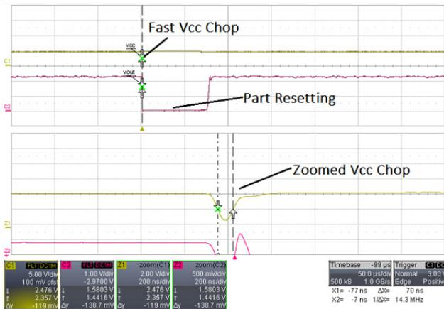
Figure 8: Device resets from V<sub>CC</sub> pulled low briefly
