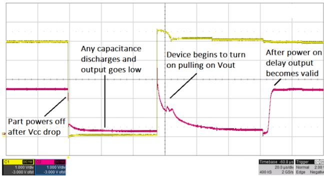
Figure 11: Normal power on and power off functionality
