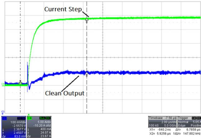
Figure 7: Perpendicular setup with minimal undershoot and ringing
