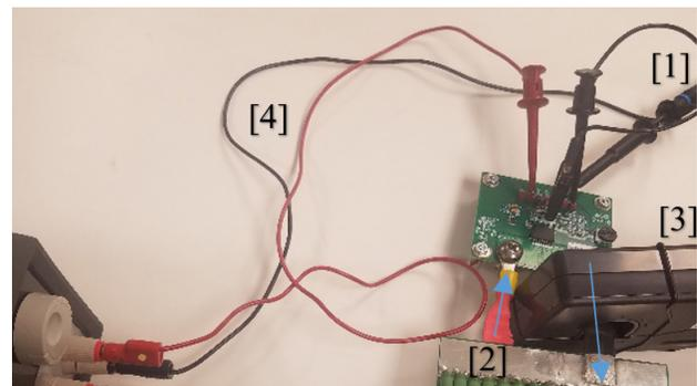
Figure 1: Poor setup allowing coupling onto  $V_{CC}$
