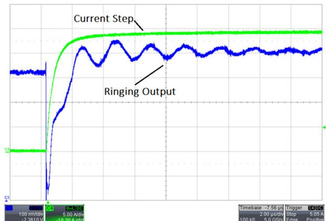
Figure 6: Parallel setup with significant undershoot and ringing
