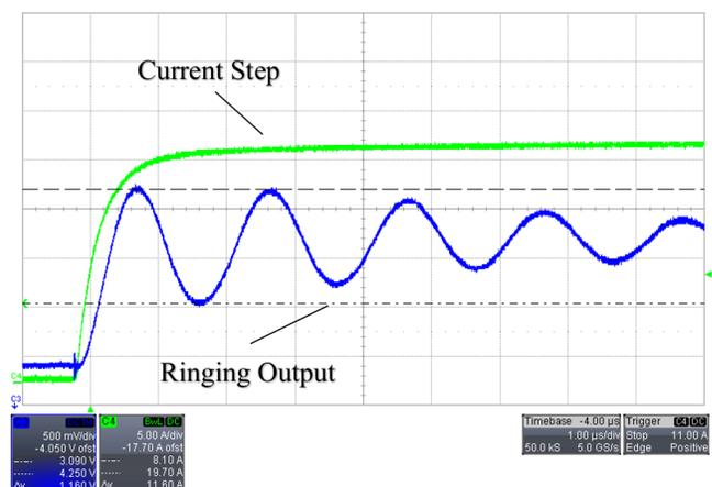
Figure 2: Poor setup output ringing
