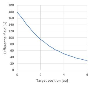
Figure 5: Typical Differential Field versus Target Position – Based on Figure 2 System
