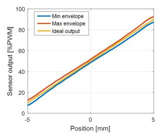
Figure 14: Sensor Output Envelope Example
