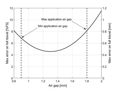
Figure 15: Typical Error versus Mounting Air Gap
