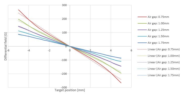
Figure 11: Differential Field Sensed by ATS344LSP Sensor versus Target Position versus Air Gap
