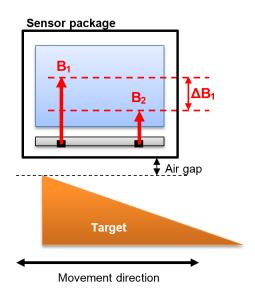
Figure 2: Basic Principle in Front of a Ferromagnetic Target – Large Differential Field When the target is moved to the left, as in Figure 3, the differential field  $\Delta B_2$  is still negative but the difference is much smaller between  $B_1$  and  $B_2$ . The reason for this change in differential magnetic field is the nonlinear behavior between the measured magnetic field level on a single Hall plate and the distance of the sensor to the target.
