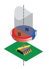
Figure 1: Sensor and magnet orientation – end of shaft
