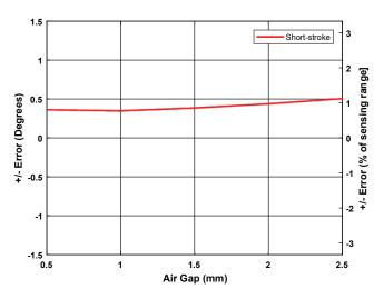
Figure 7: Short stroke accuracy error across air gap
