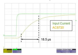
Figure 9: ACS720 Impulse Response with 4.7 nF Filter Capacitor
