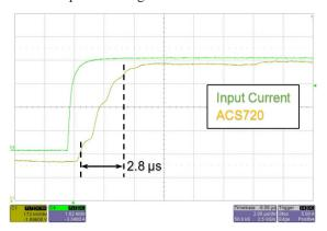
Figure 7: ACS720 Impulse Response with 0 nF Filter Capacitor
