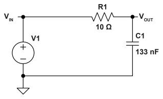
Figure 4: SPICE Model of Low-Pass Filter with Cutoff Frequency at 120 kHz
