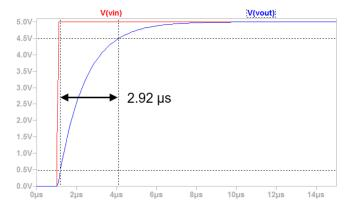
Figure 5: Impulse Response of 120 kHz Low Pass Filter
