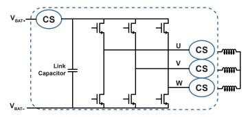
Figure 3: Simplified Three-Phase Inverter Schematic
