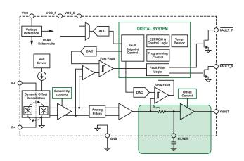
Figure 1: ACS720 Block Diagram with Emphasis on the External Filter Circuit
