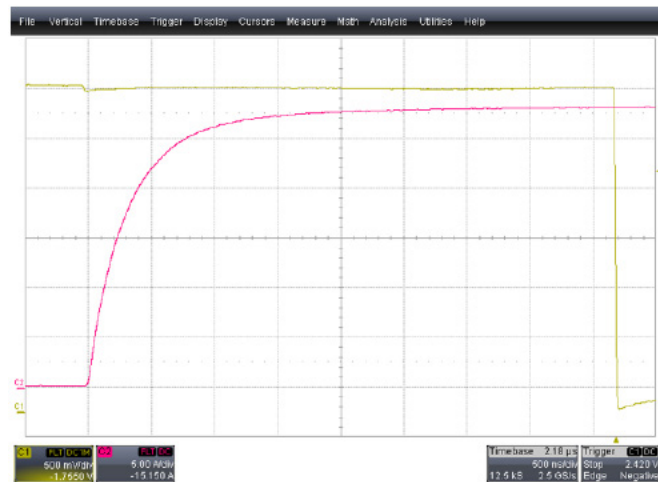
Figure 9. DIO_1 Overcurrent Fault Response with ftdly 0
