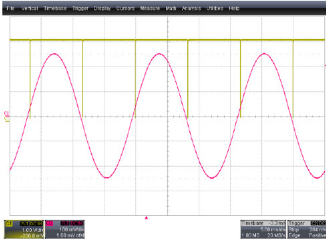
Figure 3. Voltage Zero Crossing Output with halfcycle_en Set
