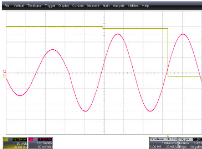
Figure 6. Overvoltage VRMS detection after 3 Half Cycle
