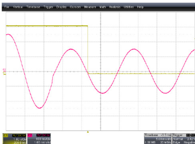
Figure 6. Overvoltage VRMS detection after 3 Half Cycle
