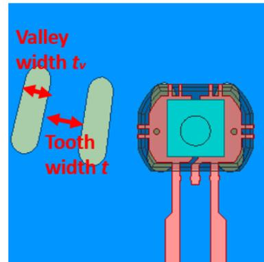
Figure 22: Definition of valley width and tooth width
