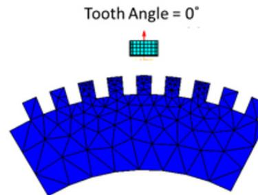
Figure 8: Example image of ferromagnetic target (blue) meshed for simulation with a tooth angle of 0°.
