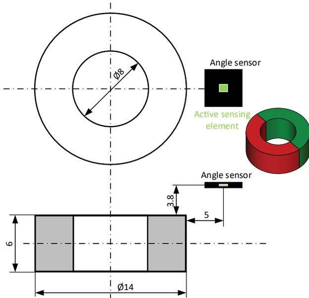
Figure 5: Side-shaft measurement, "diagonal" positioning
