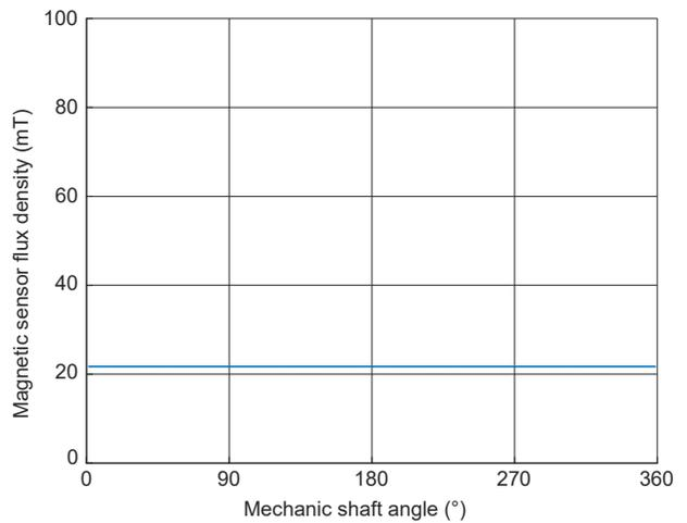
Figure 7: Side-shaft sensor signal strength, "diagonal" positioning
