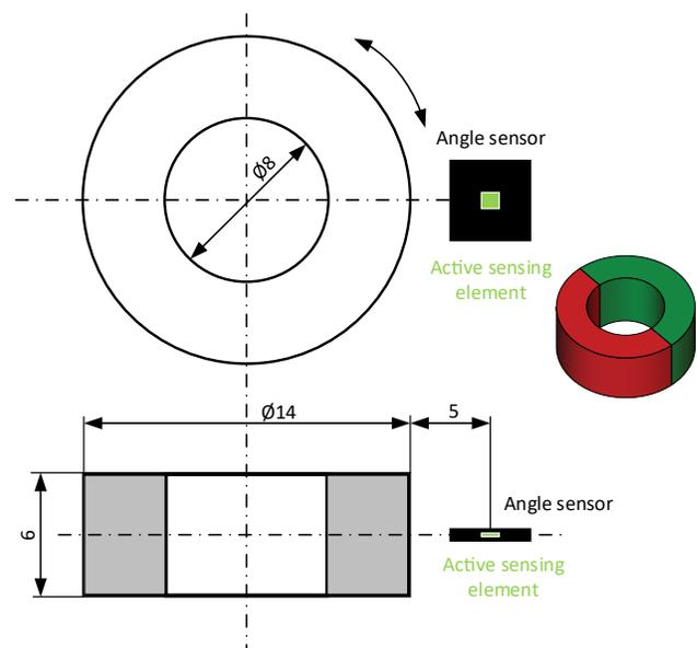
Figure 1: Side-shaft measurement, classic positioning
