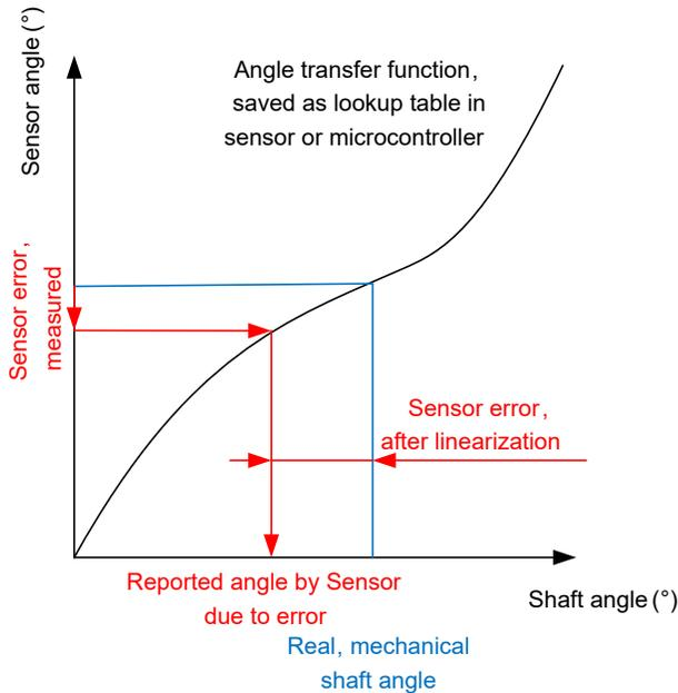
Figure 3: Sensor error amplification
