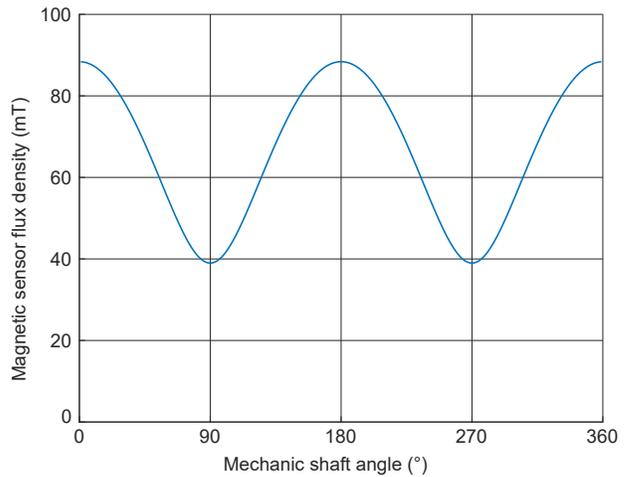
Figure 4: Side-shaft sensor signal strength (in sensor plane)
