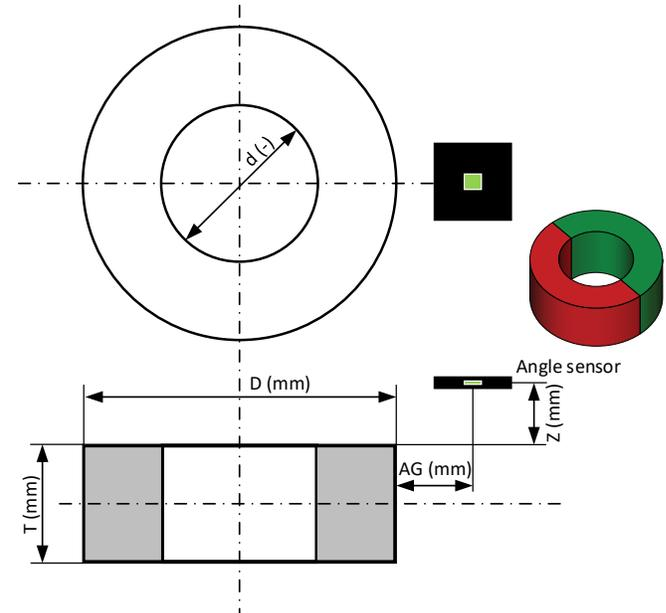
Figure 10: Variables for calculating the right position height Z
