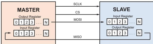
Figure 8: SPI Data Transfer
