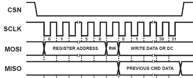
Figure 13: SPI Write Timing
