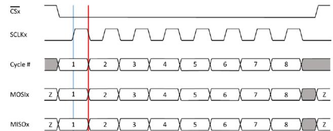
Figure 9: SPI Mode 0, CPOL = 0, CPHA = 0
