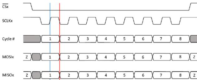
Figure 12: SPI Mode 3, CPOL = 1, CPHA = 0
