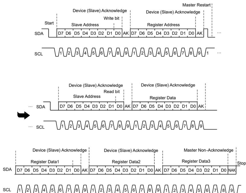
Figure 4: I<sup>2</sup>C Read Timing Diagram
