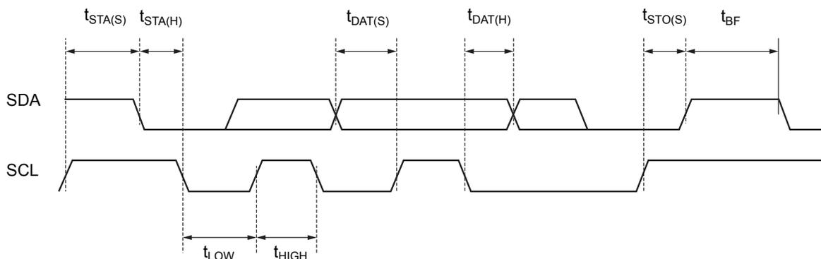
Figure 2: I<sup>2</sup>C Input and Output Timing Diagram
