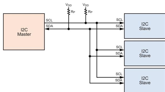
Figure 1: I<sup>2</sup>C bus diagram showing Master and Slave devices
