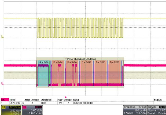
Figure 5: I<sup>2</sup>C Write Sequence
