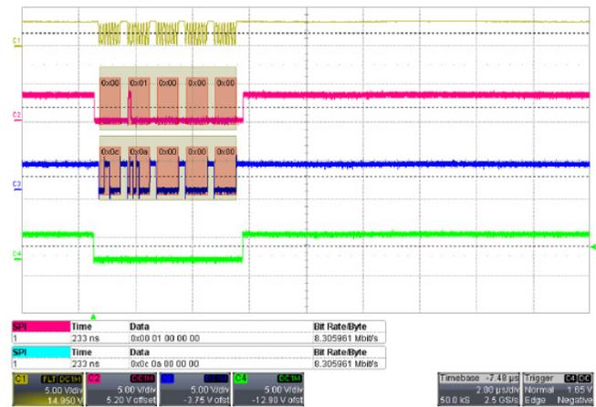
Figure 15: SPI Write Sequence
