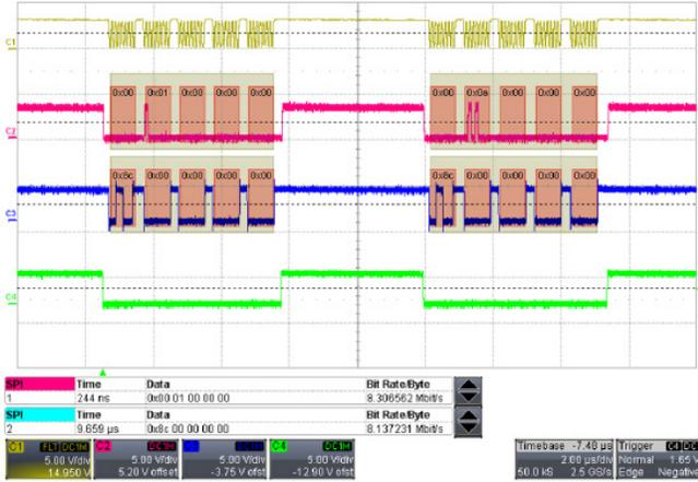
Figure 16: SPI Read Sequence
