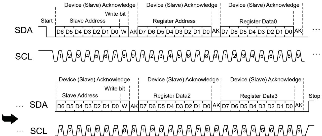
Figure 3: I<sup>2</sup>C Write Timing Diagram
