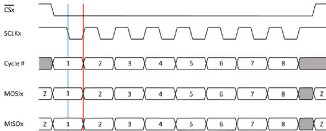
Figure 11: SPI Mode 2, CPOL = 1, CPHA = 0
