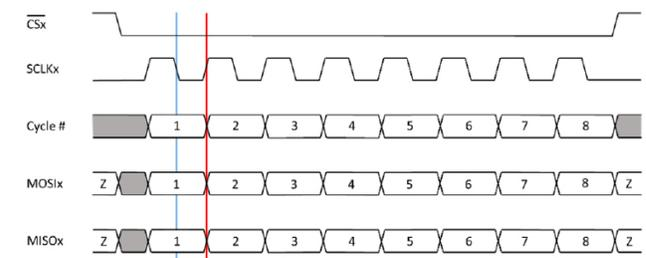
Figure 10: SPI Mode 1, CPOL = 0, CPHA = 1
