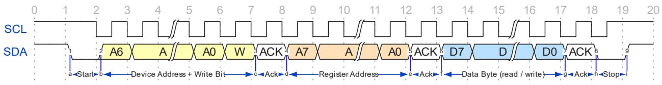
Figure 4: I<sup>2</sup>C Transmission Example
