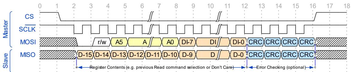
Figure 2: SPI Communication Example
