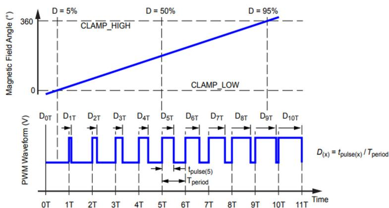
Figure 6: PWM Output Waveform and Magnetic Field Angle
