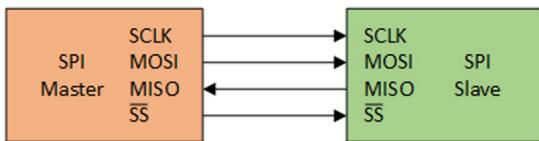
Figure 1: Basic SPI Bus Example
