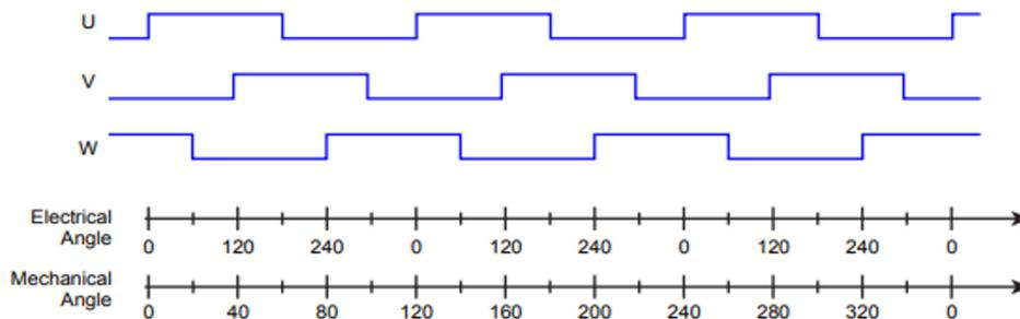
Figure 13: UVW Protocol for a Three-Pole Pair
