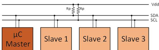
Figure 3: Basic I<sup>2</sup>C Bus Example
