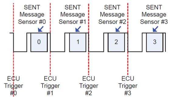
Figure 9: Sequential SENT Output Bus
