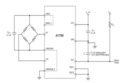
Figure 3: Typical Application Circuit of A17700 Interfaces
