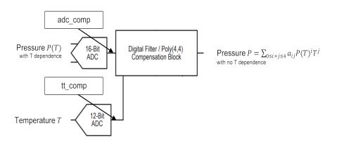
Figure 6: Digital Polynomial Compensation block inputs (Using bridge signal and temperature)
