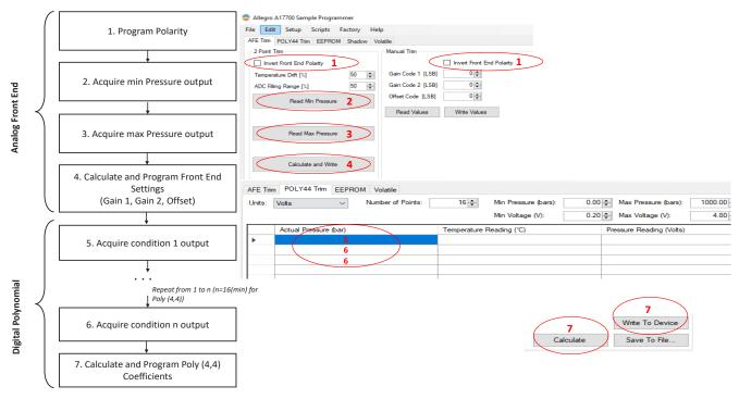
Figure 8: A17700 Compensation Flowchart and Equivalent Function On Allegro's A17700 Programming GUI
